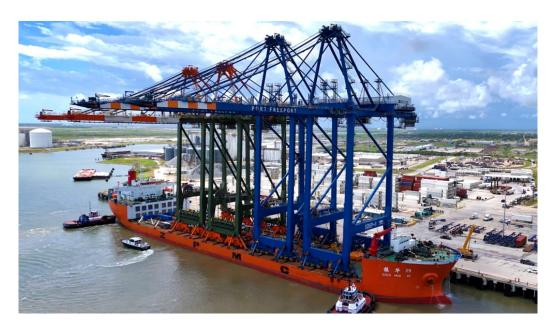
PHOTO CUTLINE: Two state-of-the-art Super Post-Panamax Gantry Cranes were delivered aboard a heavy-lift vessel, arriving at Port Freeport's Velasco Container Terminal.
