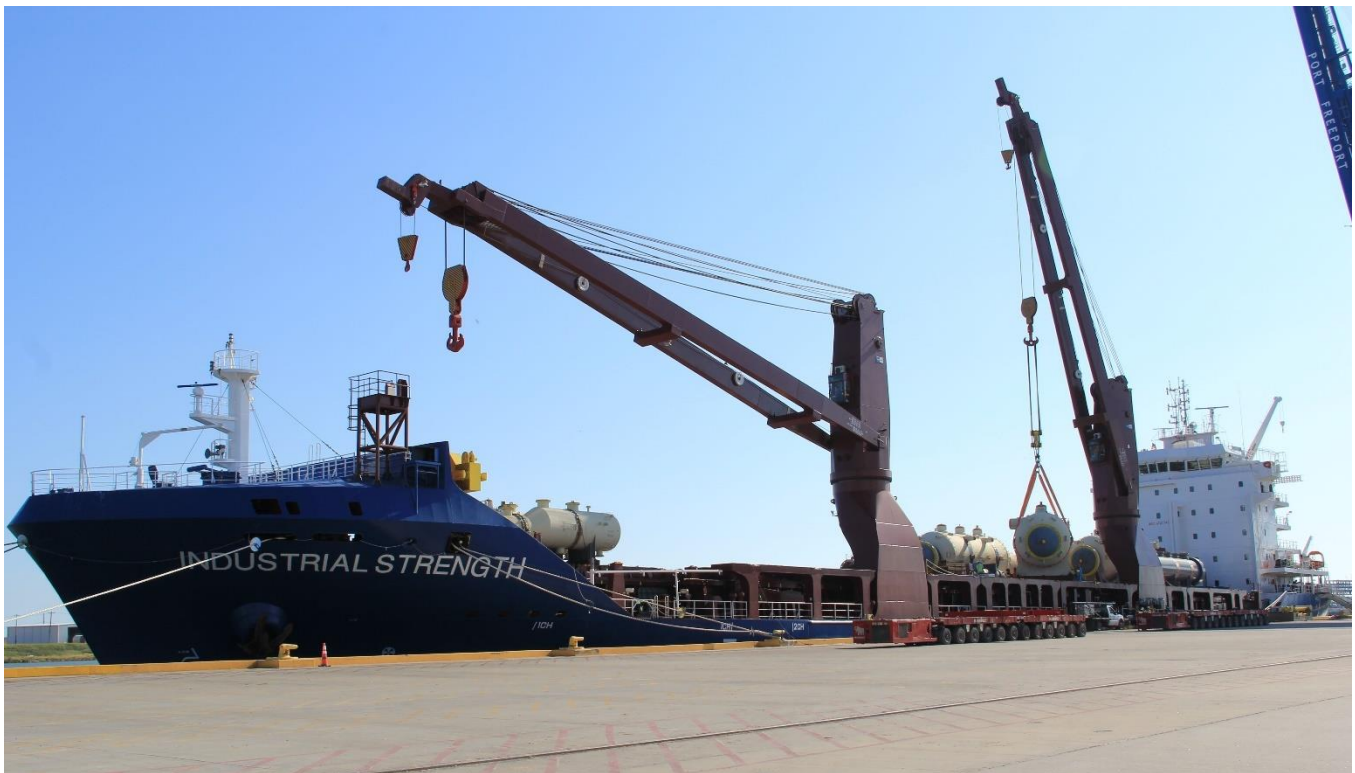
Photo 1: M/V Industrial Strength offloads propane vaporizers.
